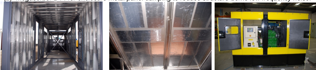
(2) Megasorber D14 for enclosure metal panel damping to reduce structure-borne low frequency noise.
