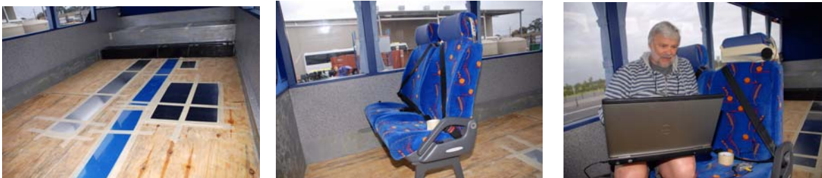
Fig 5. The noise measurement before the installation of Megasorber DIS8.
