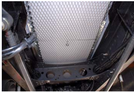
Fig 10. The installation of Megasorber FG50 with expanded metal mesh under the floor board
